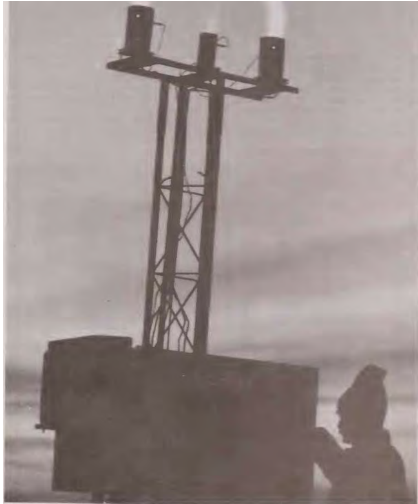
Manually operated cloud seeding generator similar to those used in the Colorado River Basin Pilot Project. (Courtesy of the Bureau of Reclamation.)
