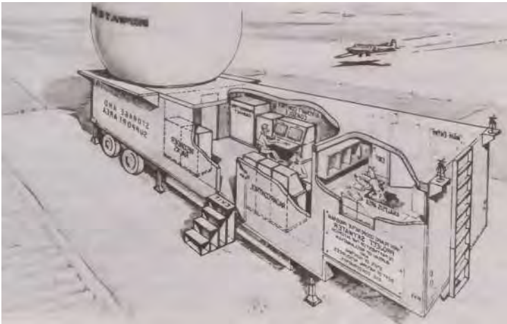
Artist's rendering of portable radar used in Project Skywater. (Courtesy of the Bureau of Reclamation.)
