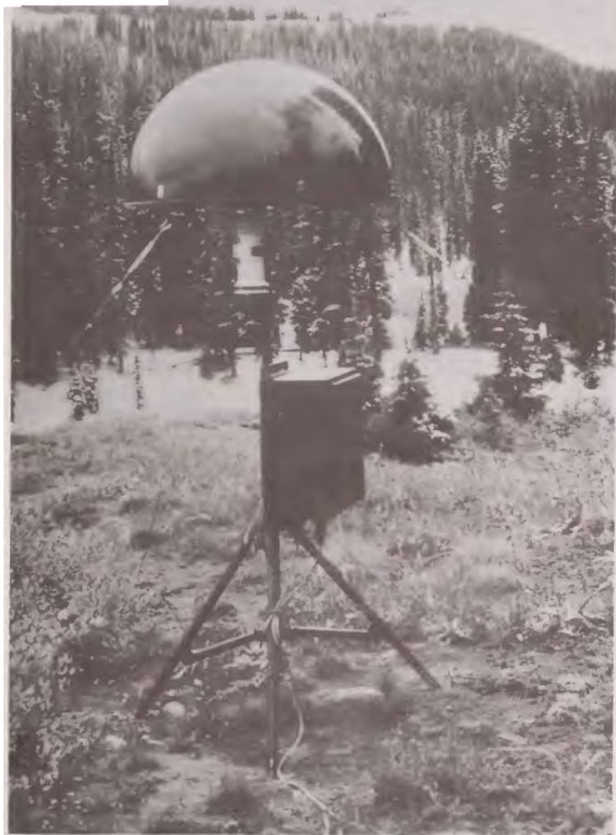
Data collection platform and transmitter used by Project Skywater in connection with the Earth Resources Technology Satellite (ERTS). (Courtesy of the Bureau of Reclamation.)
