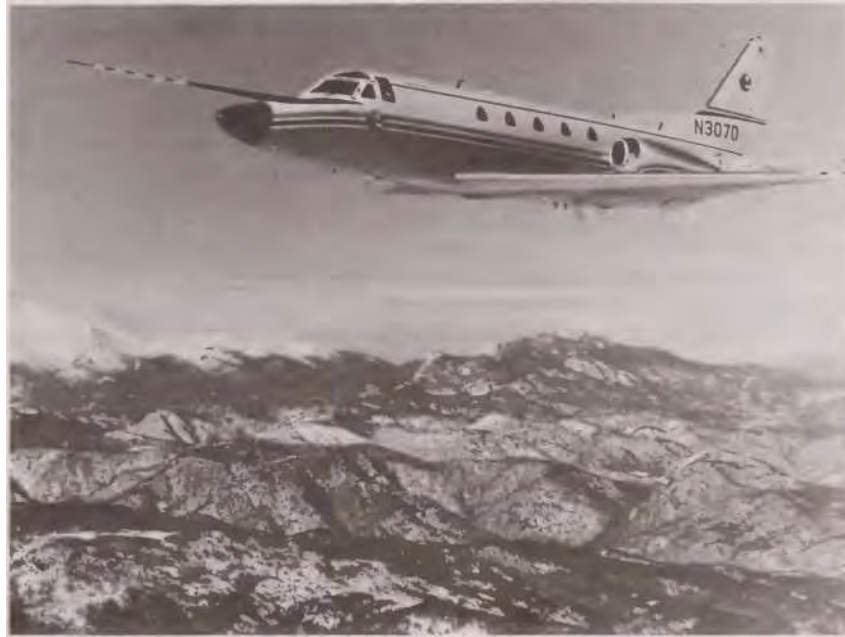
Instrumented aircraft, operated by the Research Aviation Facility of the National Center for Atmospheric Research (NCAR), whose primary mission in the 1976 summer field season of the National Hail Research Experiment (NHRE), was to assess the feasibility of on-top cloud seeding. (Courtesy of the National Science Foundation.)
